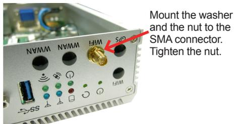
13. Have an external antenna. Screw and tightly fasten the antenna to the SMA connector.
