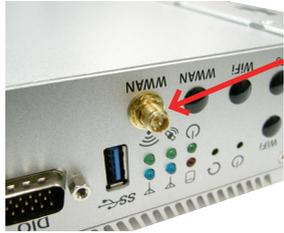
Mount the washer and the nut to the SMA connector. Tighten the nut.
