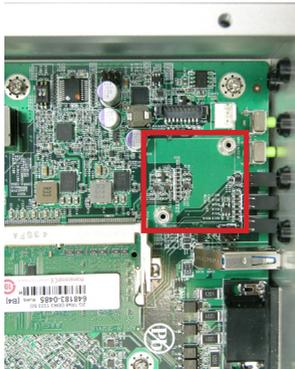
4. Fasten 2 screws to fix the module and connect the cable to the connector on the module.
