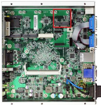
4. Prepare the **WIFI-AT2350** Wi-Fi module kit. The module is a half-size module of **PCI Express Mini-card** form factor, with two U.F.L connectors, one is "1", and the other is "0".
