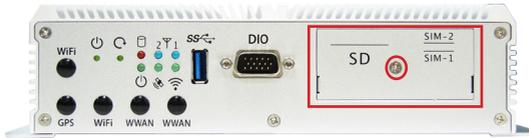
2. Slide the SD card into the slot. You can hear a slight clicking noise, which means it has locked into place.
