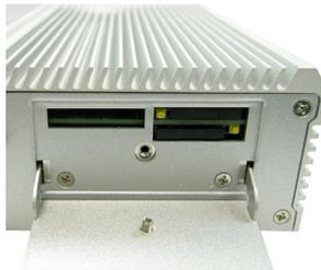
2. Use a clipper to press the eject button in the SIM card slot, and the SIM card jacket will be ejected. Pull the jacket out of the slot.
