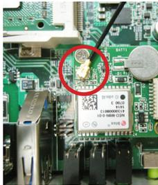
7. From the other end of the RF antenna, which is an SMA connector, remove the washer and the nut. Save the washer and nut for later use. Note the SMA connector has the form of a threaded bolt, with one flat side.
