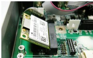
6. Press down the module and fix the module in place using two screws.
