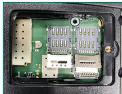
**Figure 2-7** Unlock the card slot cover(s) and insert the SIM card into the slot.
